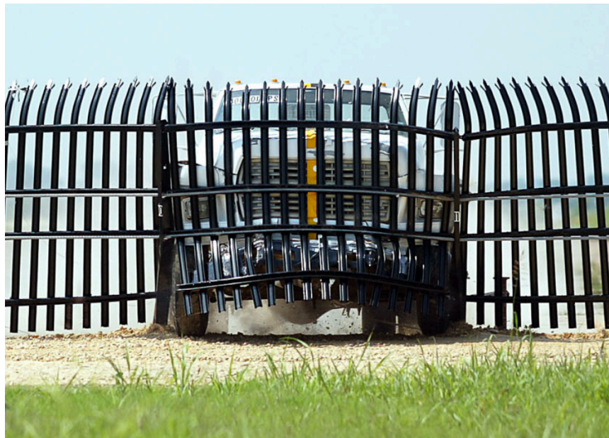
Figure 20. An illustration of a crash test for fence rating.
