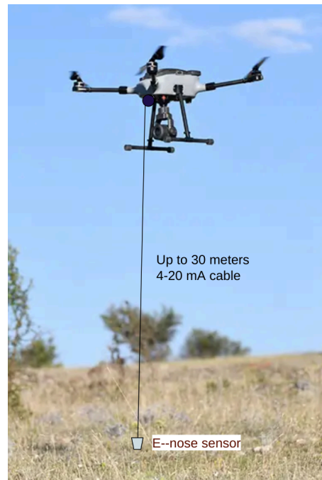
Figure 27. Illustration of vertical air sampling (Source: Author)
