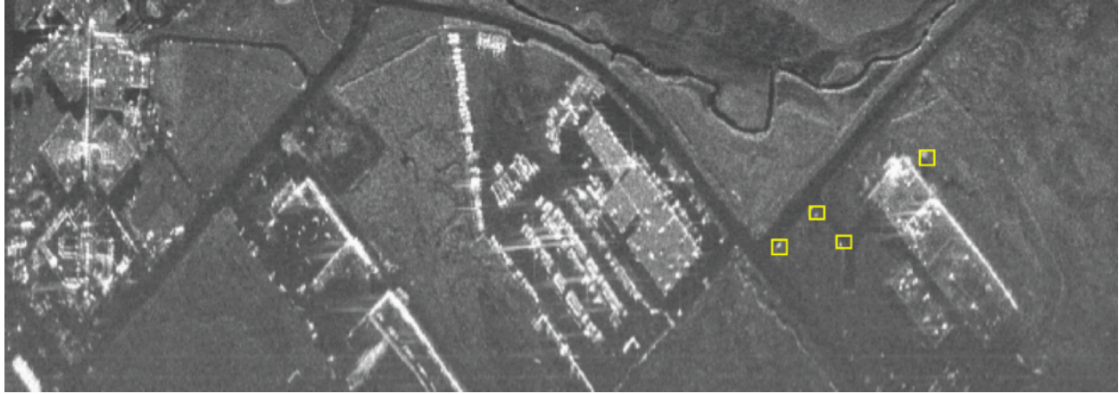
Figure 40. SAR image showing four detected humans (Source: [137])
