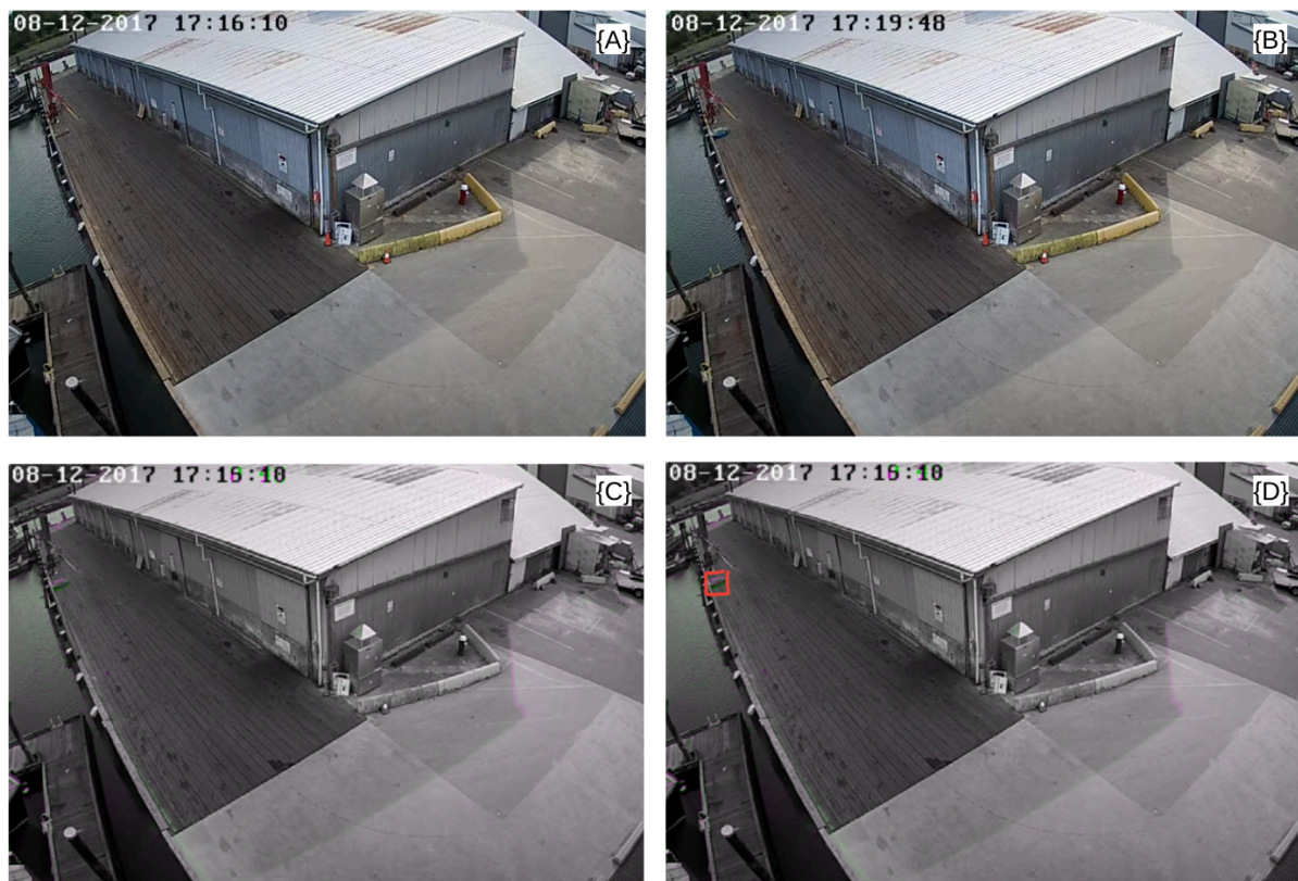
Figure 28. Detecting an object that was added to the scene during the unsurveilled period (Source: [109], processed by author)
