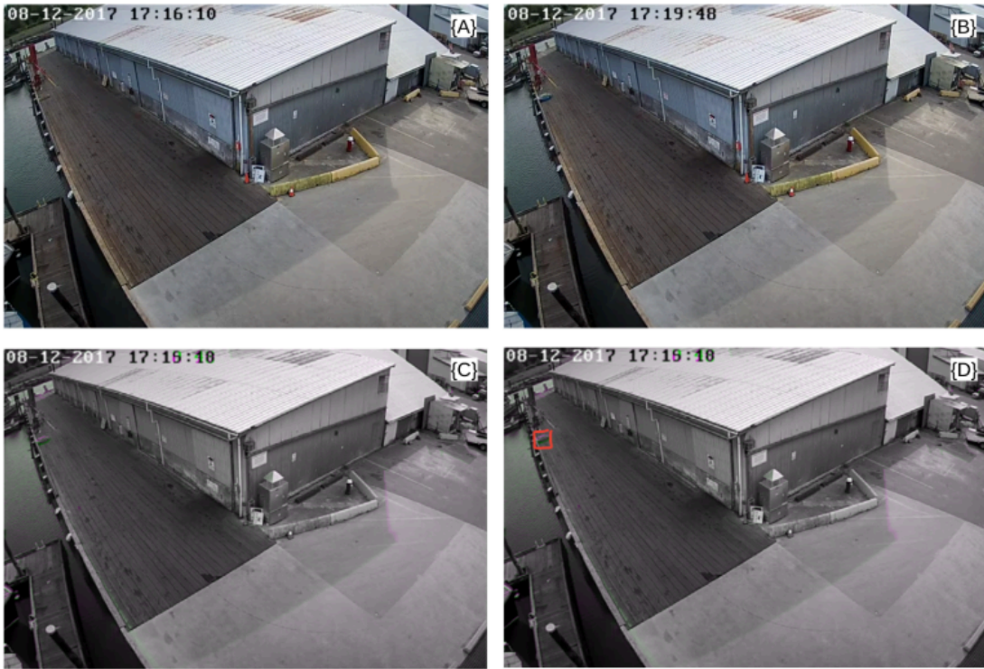
Figure 28. Detecting an object that was added to the scene during the unsurveilled period [114], processed by author
