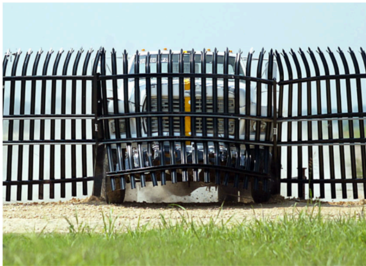
Figure 20. An illustration of a crash test for fence rating [111]
