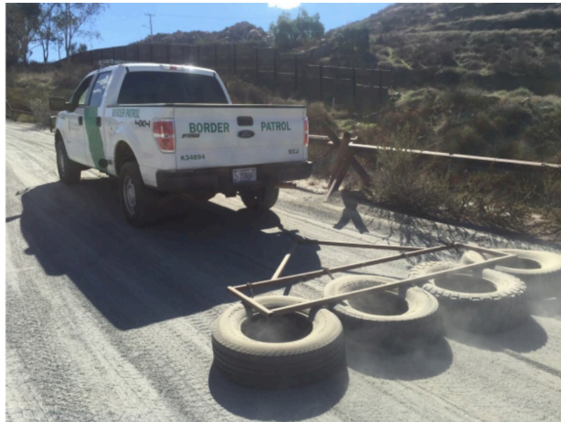
Figure 30. Refreshing the road soil so footprints show up more easily [135]
